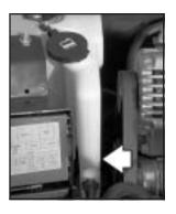
The coolant recovery tank is located between the power steering fluid reservoir and the underhood fuse block in the engine compartment on the passenger's side of the vehicle. See *Engine Compartment Overview on page 5-12* for more information on location.
